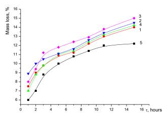
Fig. 3. The influence of the filling measure with modified montmorillonite (MM) on the isothermal mass loss of KO-08K varnish:  $1-\text{KO-08K};\ 2-\text{KO-08K+10}\ \%\ \text{MM};\ 3-\text{KO-08K+20}\ \%\ \text{MM};$   $4-\text{KO-08K+30}\ \%\ \text{MM};\ 5-\text{KO-08K+40}\ \%\ \text{MM}$
