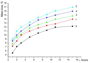
Fig. 2. The influence of the filling measure with modified palygorskite (MP) on the isothermal mass loss of KO-08K varnish:  $1-\text{KO-08K};\ 2-\text{KO-08K+10}\ \ \text{MP};\ 3-\text{KO-08K+20}\ \ \text{MP};$   $4-\text{KO-08K+30}\ \ \text{MP};\ 5-\text{KO-08K+40}\ \ \text{MP}$
