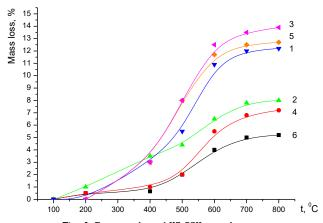
Fig. 4. Derivative loss of KO-08K varnish mass:
