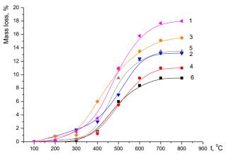
**Fig. 6.** Derivative loss of KO-978 varnish mass: 1 – KO-978; 2 – KO-978 after heat treatment; 3 – KO-978+MP; 4 – KO-978+MP after heat treatment; 5 – KO-978+MM; 6 – KO-978+MM after heat treatment
