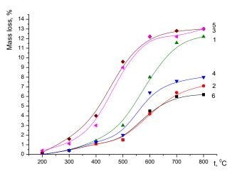
**Fig. 5.** Derivative loss of KO-921 varnish mass: 1 – KO-921; 2 – KO-921 after heat treatment; 3 – KO-921+MP; 4 – KO-921+MP after heat treatment; 5 – KO-921+MM; 6 – KO-921+MM after heat treatment
