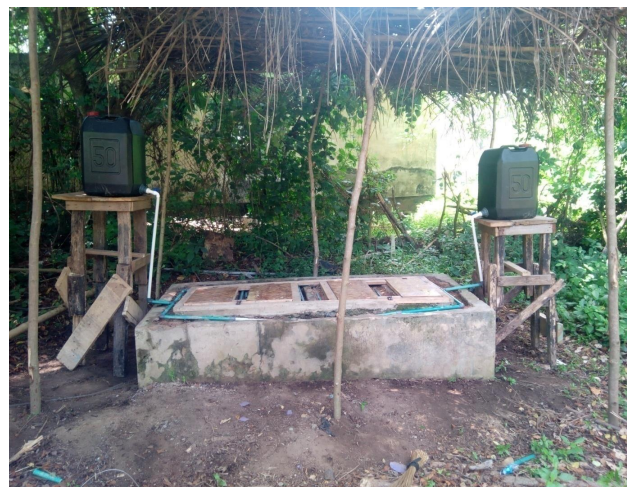
Fig. 1. Evaporative cooling chamber with water reservoir
