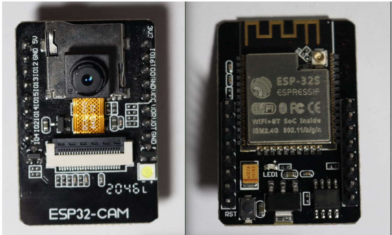
Figure 5: ESP32-CAM AI-THINKER MODULE (Source: authors)
