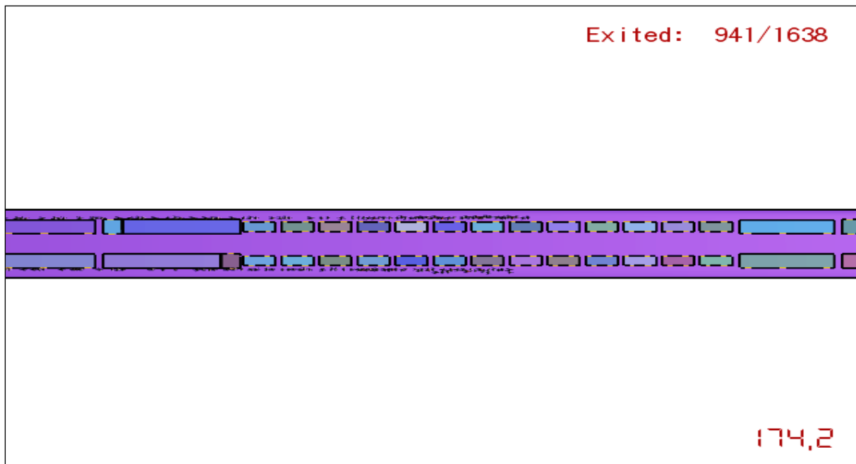
Figure 2: The collision in the middle of the tunnel after 174.2 seconds for the first scenario (Source: Jevtić, B. R. (2016) Evacuation from tunnels-an example of Straževica tunnel)
