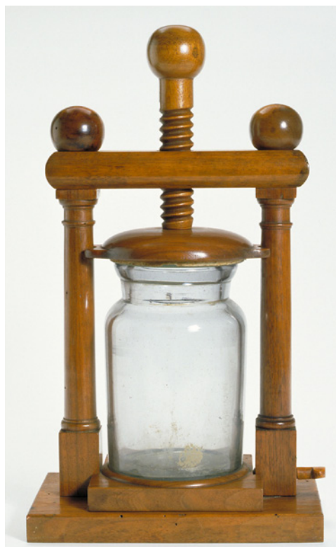
FIGURE 4.1 A large disinfection apparatus for military hospitals and other public spaces. Museo Galileo's Photographic Archives: Pressure receiver (Inv.3778). COURTESY OF MUSEO GALILEO, FLORENCE.
