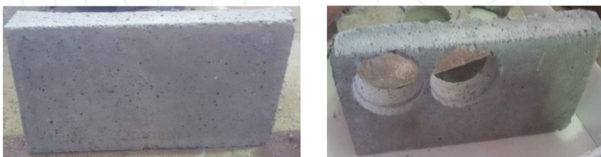
Figure 2. Sample of plastic cement produced in this research with a hole [10].
