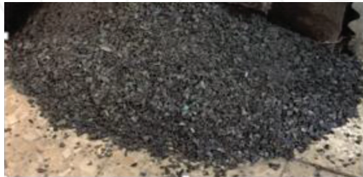
Figure 1. Polyethylene waste after cutting and grinding [10].
