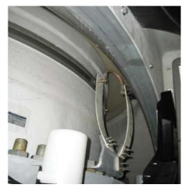
Figure 3.2 Lightning current transfer unit, LCTU
