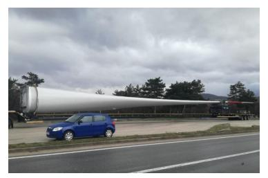
Figure 3.1 V112 model blade on the ground during transport
