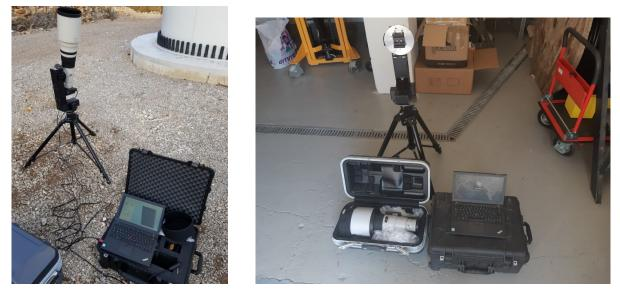
Figure 5.1 Mounted equipment prepared for recording (zoom on one of the blades)
