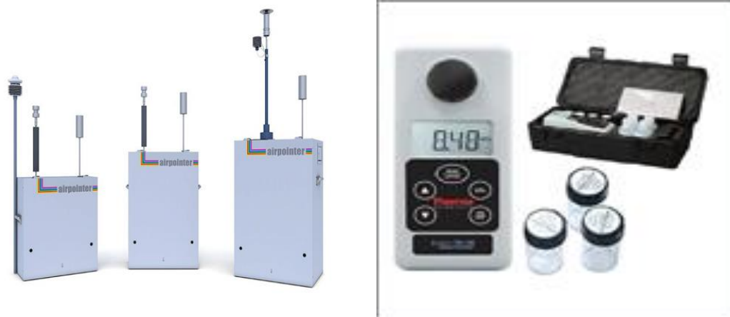
Figure 1: Air Pointer (system for air quality monitoring); Infrared Turbidimeter (designed for quick and easy turbidity measurement) (Source: https://www.znrfak.ni.ac.rs )
