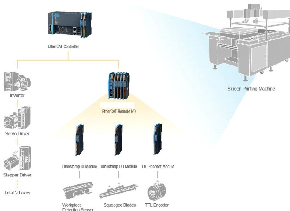
Fig. 5. Scheme of computer control of screen printing based on the distributed architecture «EtherCAT» [16]
