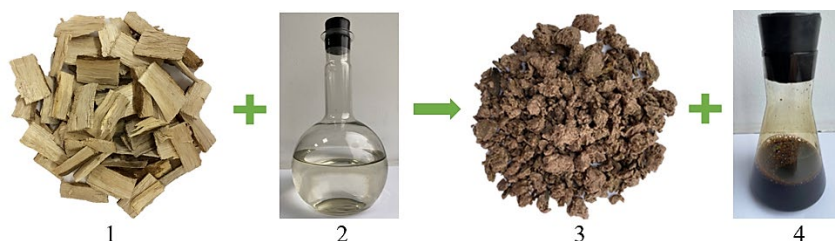
Fig. 1. The general scheme for obtaining fibrous semi-finished products and black liquor: 1 – wood chips; 2 – sodium chloride; 3 – washed fibrous semi-finished product after cooking; 4 – black liquor
