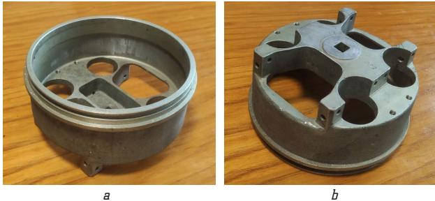
Fig. 1. AE steering machine body: a – inner side; b – the outer side
