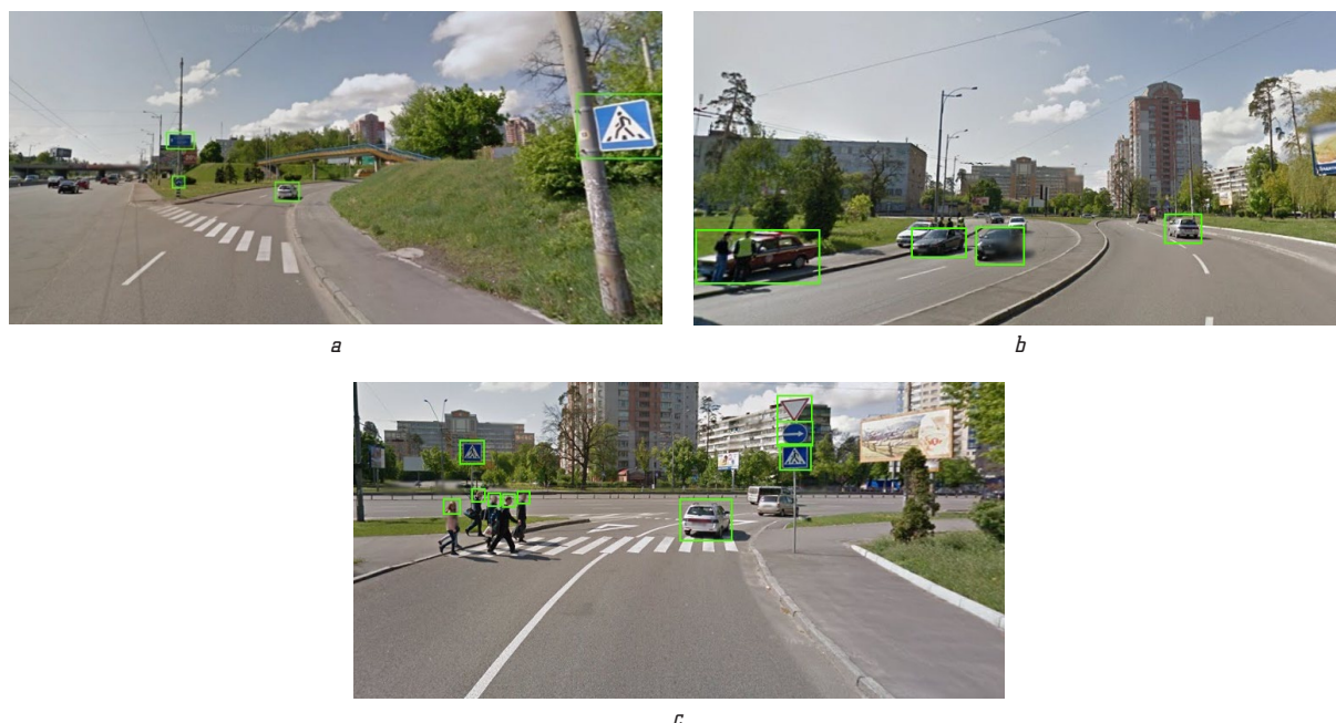
Fig. 8. Recognition and identification: a – vehicles and road signs before driving in the direction from the Great Ring Road to the Zhytomyr highway; b – recording of road accidents involving motor vehicles; c – road signs, vehicles and people
