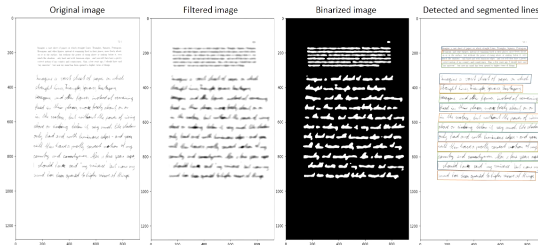
Fig. 1. The basic workflow of the text segmentation task. Filtering and binarization are one of possible preprocessing steps before the segmentation process. The result of handwriting segmentation can be presented as bounding boxes of the segmented text lines
