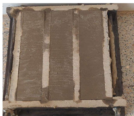
Fig. 4. Mold for making test specimens
