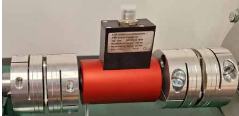
Figure 6 Torque sensor Dataflex 16/50 with steel laminae coupling Radex NC26
