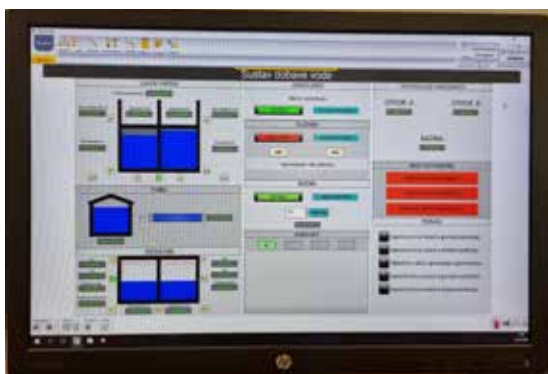
Figure 6 Water supply system – main display
