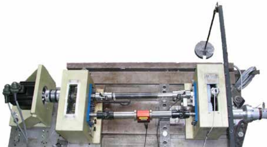
Figure 3 Mechanically closed loop polymer gear testing rig [7]
