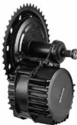
Figure 1. “Bafang” central motor with transmission gear
