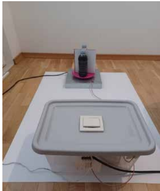
Figure 2 Assembly for simulating a bottle filling line
