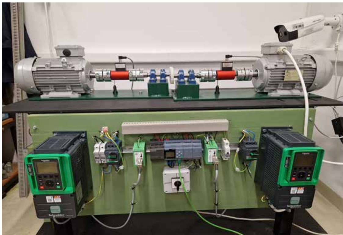
Figure 10 In-house assembled non-mechanically closed loop test rig for polymer gears
