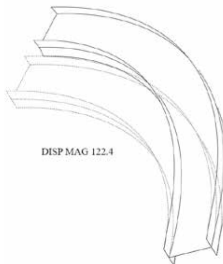
Figure 7 Deformed and undeformed (dashed line) configuration of the finite shell model of a curved beam with moderate curvature
