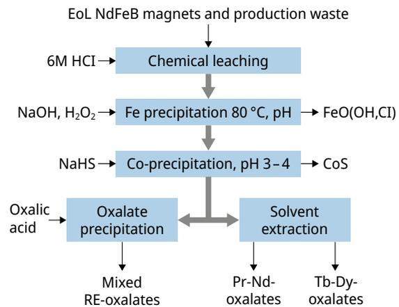
**Fig. 6: Example of a hydrometallurgical recycling process for NdFeB magnets. Own chart based on ELWERT et al. (2017)**
