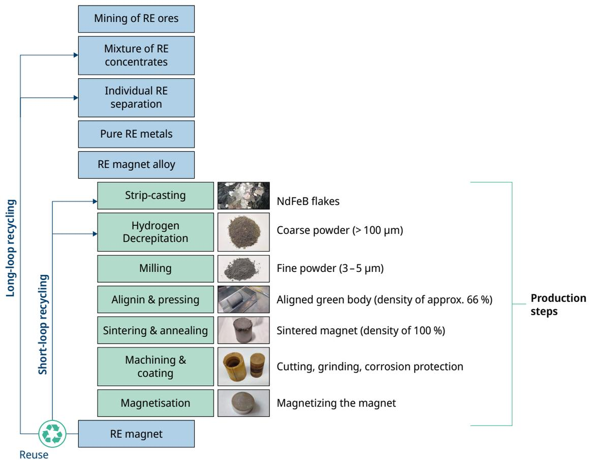
**Fig. 3: Value creation, production steps and different recycling methods in NdFeB sintered magnet production. Own graph, partly based on GAUB & GUTFLEISCH (2016). Given the high oxygen affinity of rare earths, the process steps from strip-casting through sintering and annealing are conducted in an inert gas atmosphere or vacuum**
