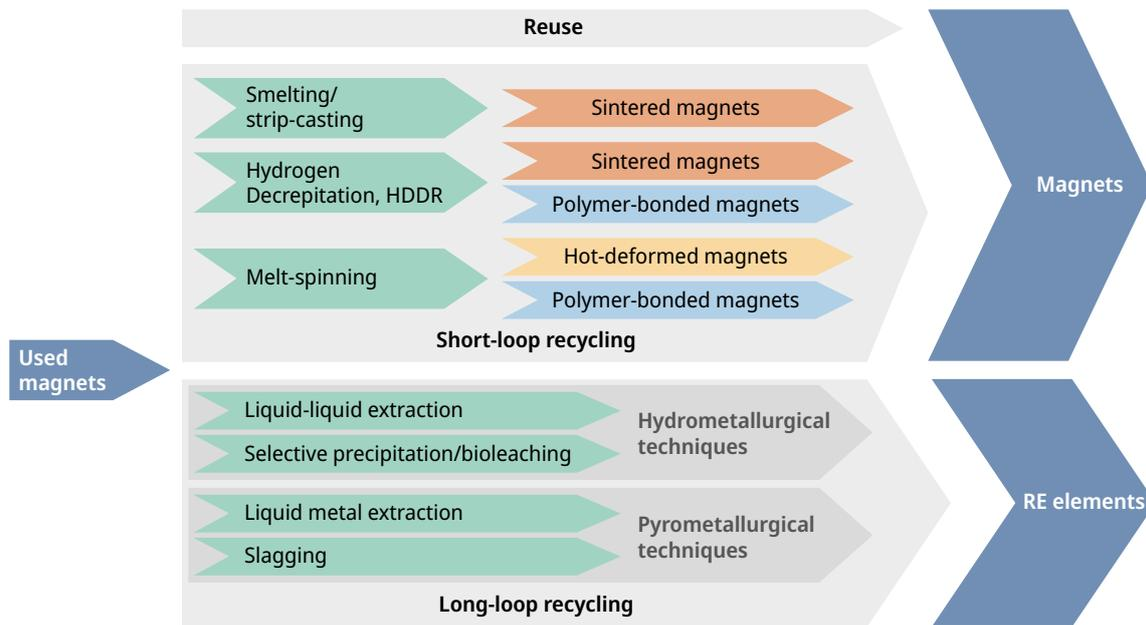
**Fig. 8: Possible recycling techniques for used magnets or production waste with the technologies used. Own chart based on GAUB et al. (2015)**
