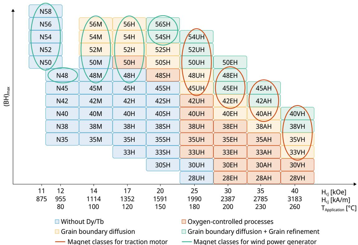
**Fig. 9: Commercially available NdFeB magnet grades with details of typical magnetic parameters and operating temperatures. Own graph based on FURGERI (2020), on the basis of the Chinese standard GB/T 13560-2017 (2018). The colour coding represents the technical development of NdFeB magnets with the aim of achieving increasingly better or higher coercive field strengths and thus developing applications with higher temperatures, such as traction motors**
