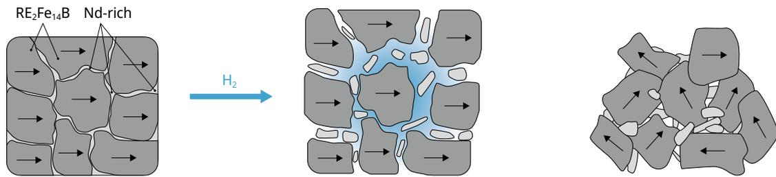
**Fig. 4: Schematic diagram showing how hydrogen decrepitation works. Own graphic based on GAUß et al. (2015)**
