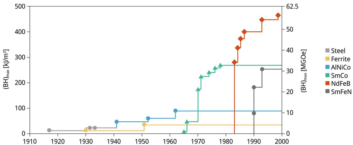
Fig. 1: Energy density  $(BH)_{\max}$  in  $\text{kJ}/\text{m}^3$  and MGOe for different permanent magnet materials and their historical development. Own graph based on GUTFLEISCH et al. (2011)
