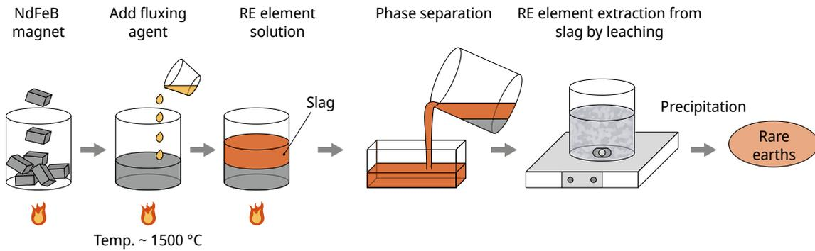
Fig. 7: Example of a pyrometallurgical recycling process for NdFeB magnets. Own illustration based on KUMARI & SAHU (2023)
