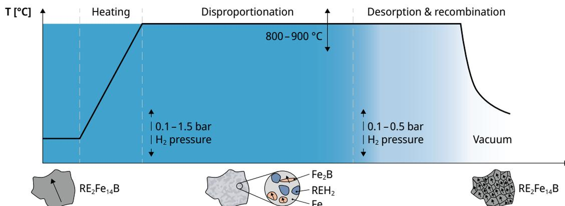
**Fig. 5: Process diagram showing the HDDR method and resulting polycrystalline microstructure. Own diagram based on GAUß et al. (2015). During disproportionation, the  $\text{RE}_2\text{Fe}_{14}\text{B}$  phase is broken down and reassembled (recombination) after desorption (outgassing of  $\text{H}_2$ ). This transforms the microstructure from monocrystalline grains into a finer polycrystalline microstructure**
