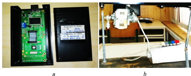
Fig. 2. Additional body equipment: a – accelerometer; b – device for creating vibrations
