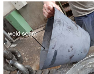
Fig. 5. Preparation for forming a «Stator housing» part: a – semi-die; b – workpiece
