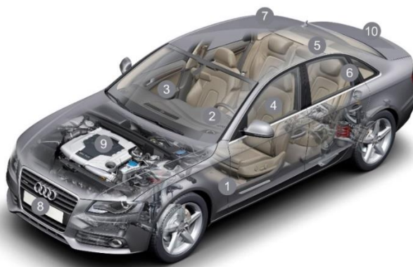
Figure 3: Car parts made of natural fibre composites
